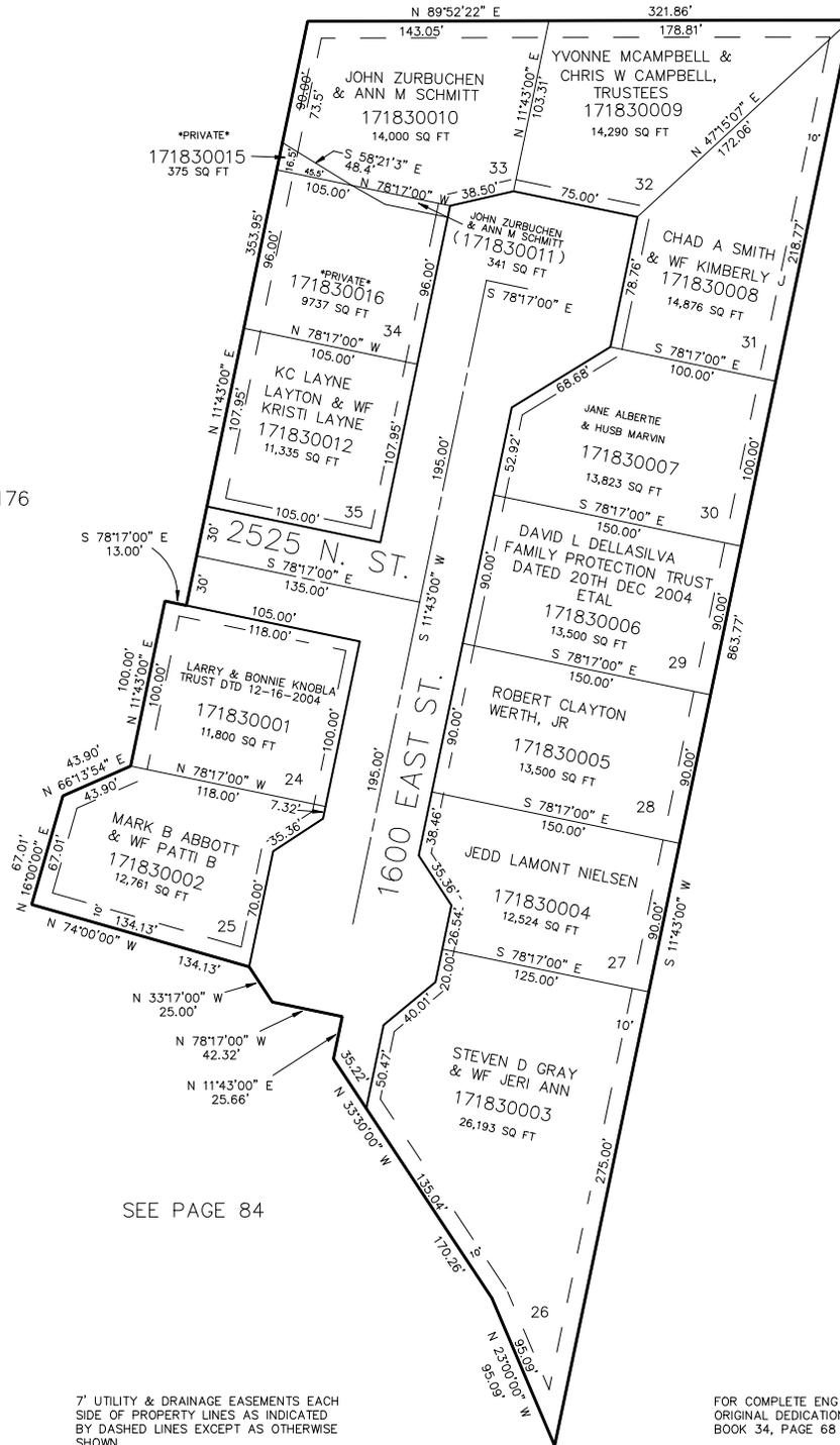
7' UTILITY & DRAINAGE EASEMENTS EACH SIDE OF PROPERTY LINES AS INDICATED BY DASHED LINES EXCEPT AS OTHERWISE SHOWN.
